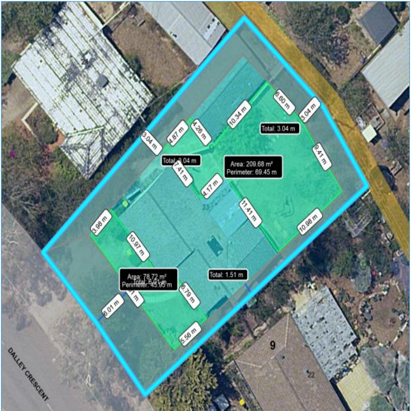
Aerial View of the Project Block with Building Offsets and Building Zone
